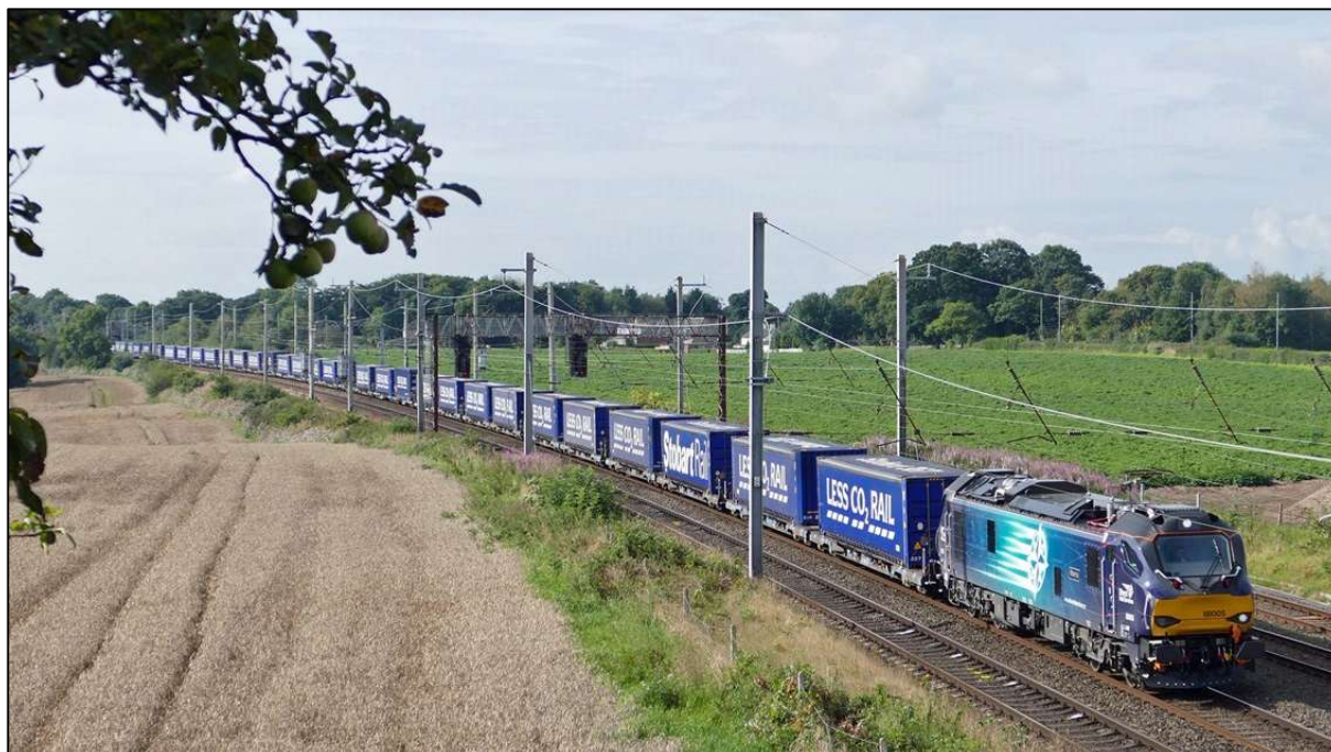
Figure 7 Train operated for Tesco conveying 8'6" and 9'6" high containers on low-height wagons (source Network Rail)
