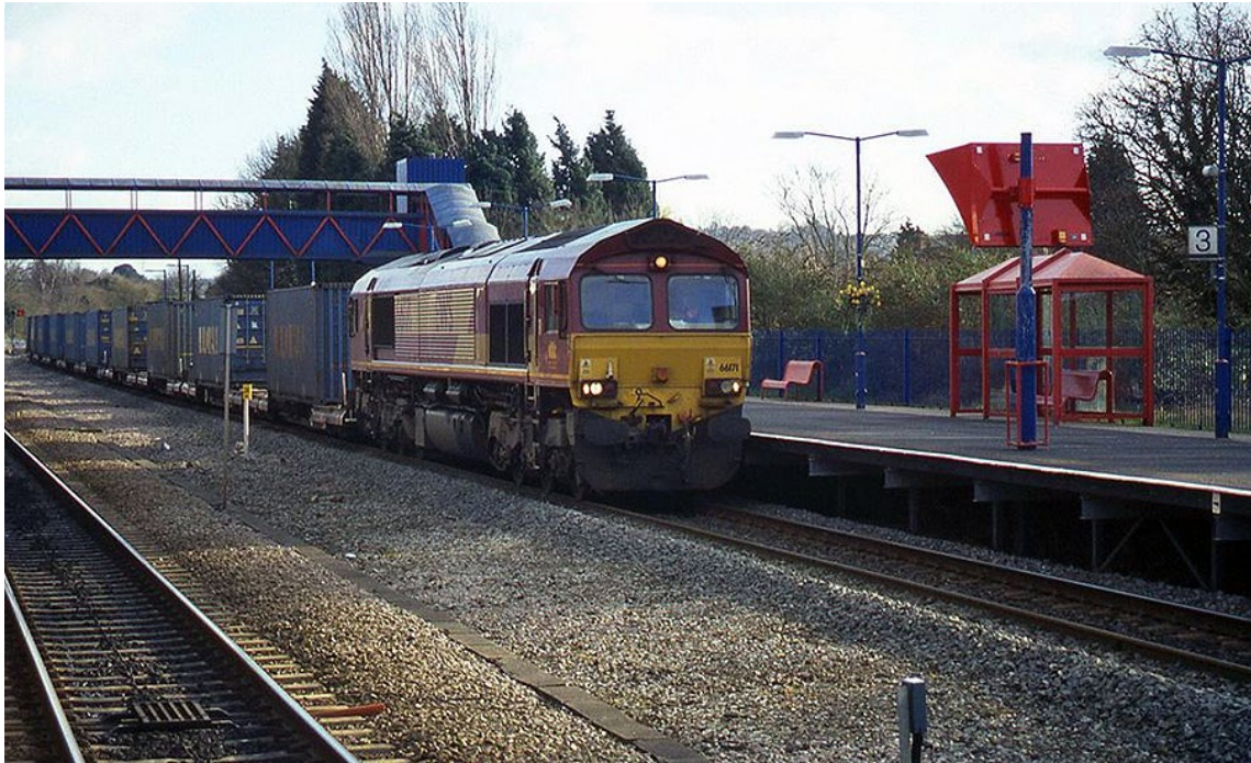
Photo: Class 66 hauling swap bodies on FKA Megafret wagons on the Chiltern Main Line at Princes Risborough (Wembley to Manchester via High Wycombe and Bicester), March 2008 © 2008 djipix.com
